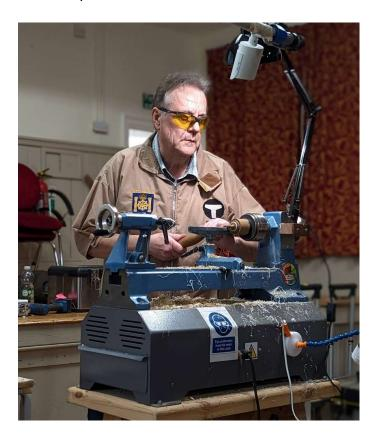
Gary started by demonstrating some basic cuts with the common turning tools, before putting them into action to turn three interesting items for us. The first was a small box with finial, made from "Mexican Rosewood", a.k.a. Bocote. Gary demonstrated a technique he described as an "onlay", using a piece of Corian, and explained that it was a quicker and easier alternative to making a traditional inlay, and the result is essentially the same, leaving a ring of contrasting material glued in place.
